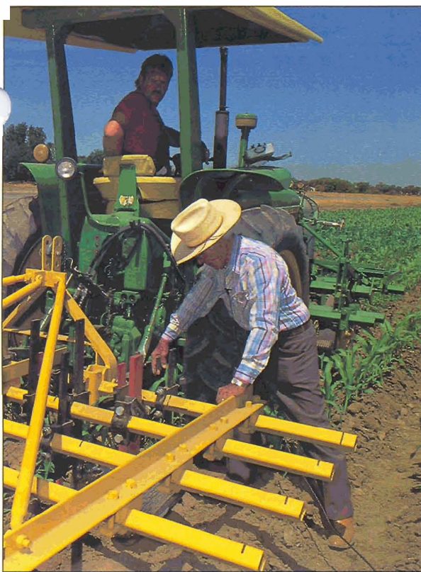
An in-row cultivator uproots weeds in the organic corn plots. The torsion rods loosen soil in the crop row, dislodging small weeds without injury to the deep-rooted corn crop.
