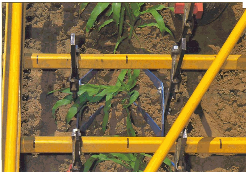
An in-row cultivator uproots weeds in the organic corn plots. The torsion rods loosen soil in the crop row, dislodging small weeds without injury to the deep-rooted corn crop.
